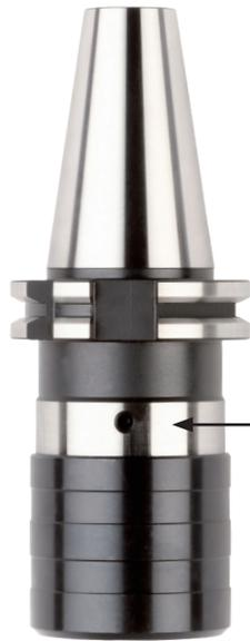
Adjustment screw for amplification of chamfer edge pressure. Turning the screw clockwise amplifies the chamfer edge pressure.
