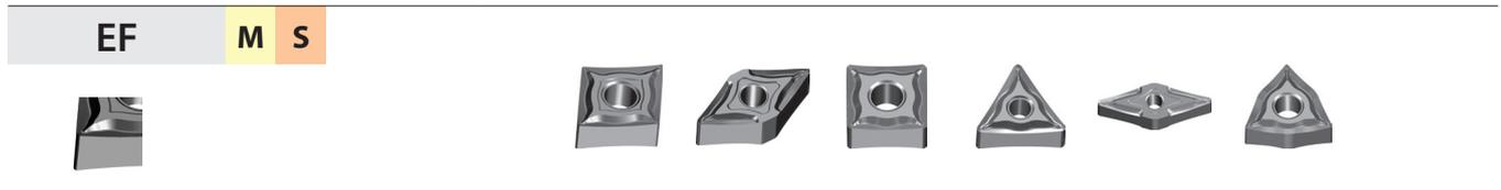
Double sided chip breaker with sharp cutting edge and large rake angle for finishing of stainless steel.
