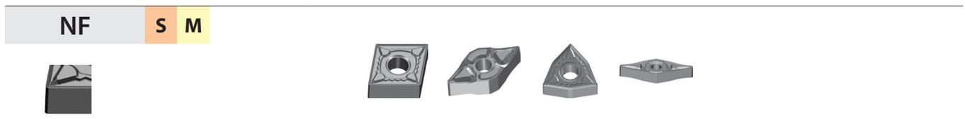
Double sided chip breaker with ground cutting edge and large rake angle for finishing. E-tolerance for high repeatability.
